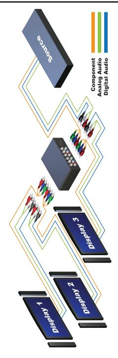
Component cable maximum distance is 50 feet at 1080p resolution without a COMP-CAT5-EXT
